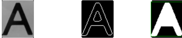
Fig. 2 (a&b) Gray scale image& noise free image (c) Highlighted edges (d&e) Filled holes & bounded box
